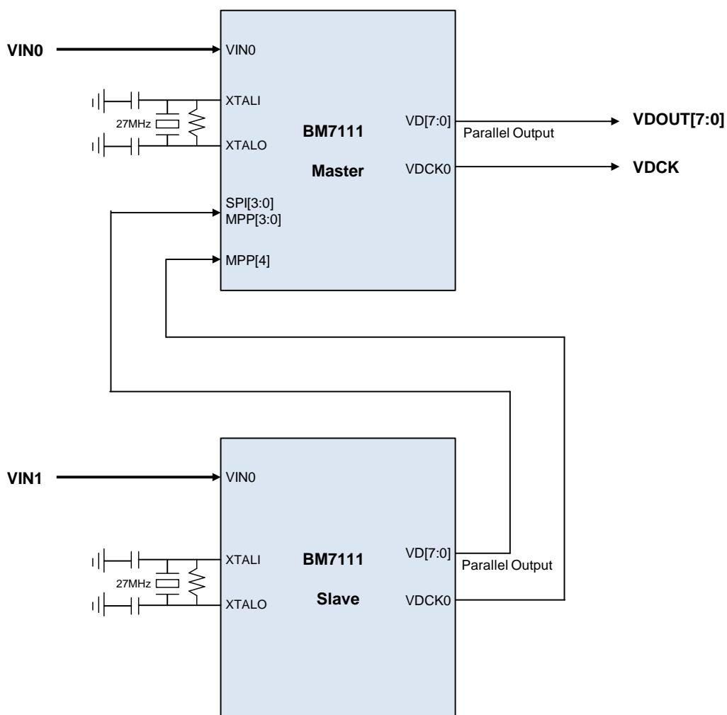
**Fig 6. Cascade Connection for Multi-chip Application**
