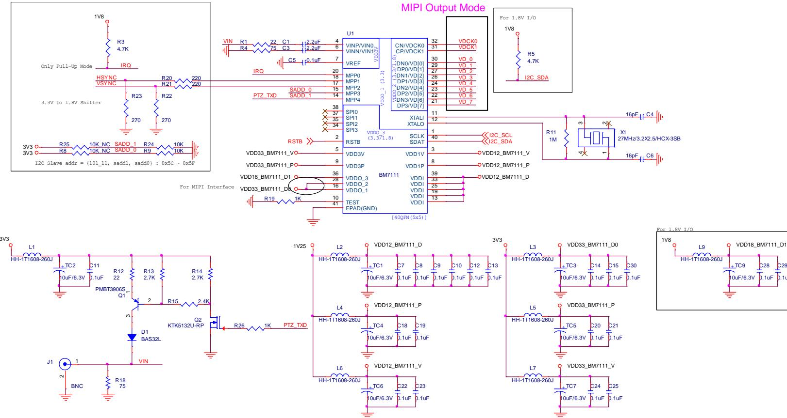
**Fig 9. Reference Schematic of 1.8V IO Supply Application for MIPI Output Mode**
