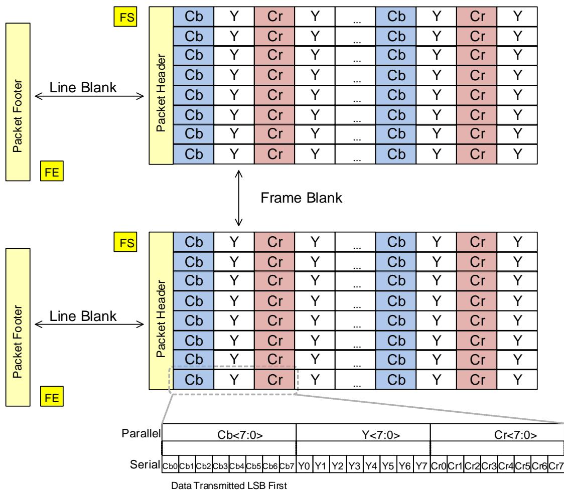
Fig 3. YUV422 8 Bit Frame Format for MIPI Transfer
